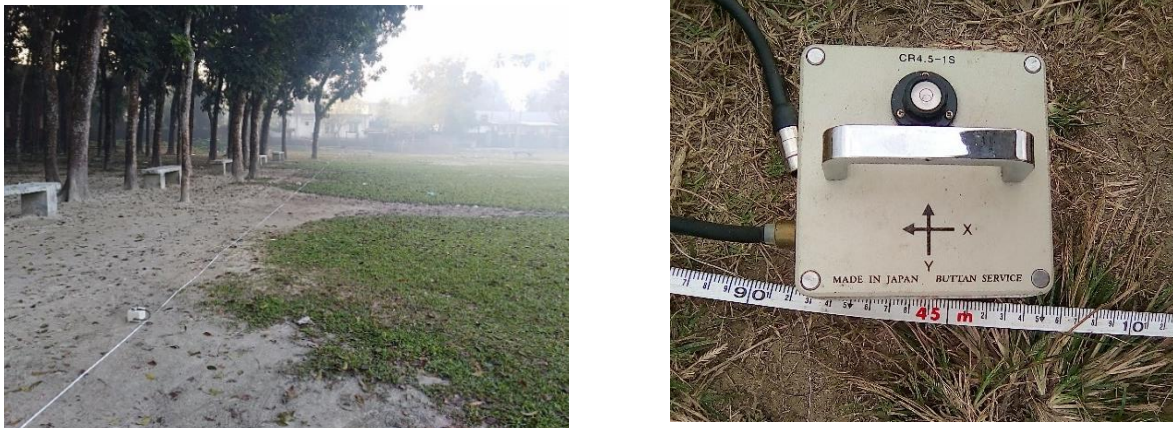
Figure 3.3: Setup of sensor for microtremor test
